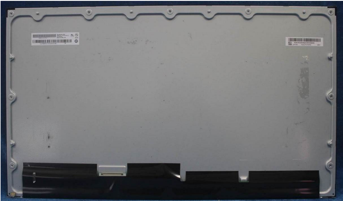
S7. Remove the Mylar and unscrew the all of the screws to remove the power board, main board from mainframe
